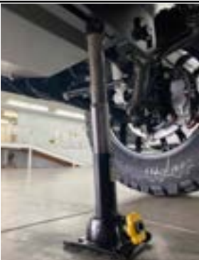
Example of jack placement on outboard end of added cross-member.
